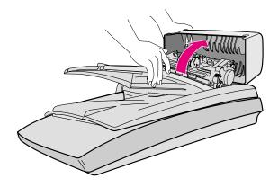
**2** Lift the large green tab (located to the left of the roller) and gently remove the jammed page.
